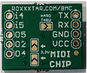
You can also use MIDI as a way to communicate via Serial between boards with different logic levels, for example: a Teensy (at 3.3v) and an Arduino Uno (at 5v), in cases like that one you can wire your boards like this:
